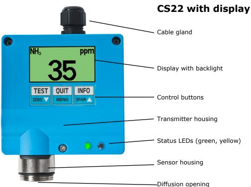
The gas sensor and the transmitter electronics are installed in the transmitter housing. The electronics converts the measuring signal into a gas concentration and transmits it either by means of an analogue current signal of 4-20mA or 0.2-1mA or a digital RS485 bus signal according to the Modbus RTU protocol. In the variant with display, gas concentration and status information are shown on the device.
