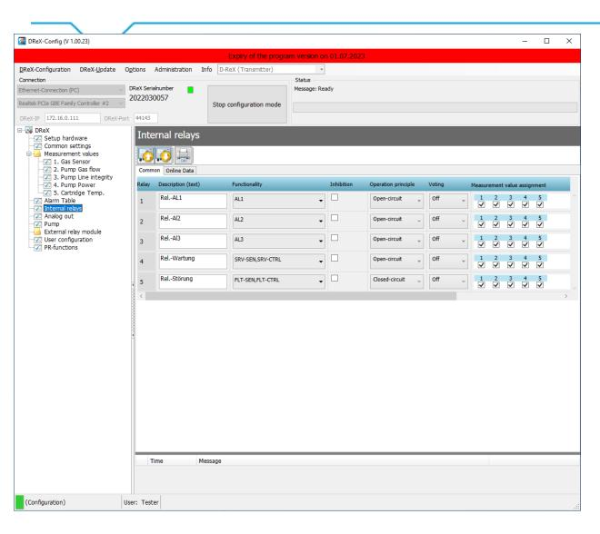
Menu for configuring and assigning the internal relays.
