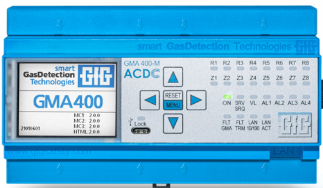
GMA400 – with Modbus TCP and web access via ethernet
