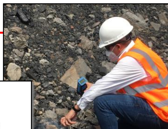
G460 instrument 1, sample from coal seam gas vent, readings for PID (isobutylene scale), and H 2 S
