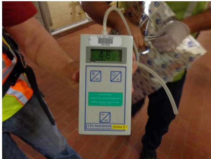
Selective NDIR detection of \text{CO}_2 ( \lambda \approx 4.3 \mu\text{m} )
