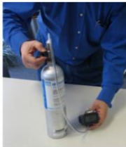
Figure 1. Performing a functional "bump test" by exposing the instrument to test gas takes only a few moments to perform.
