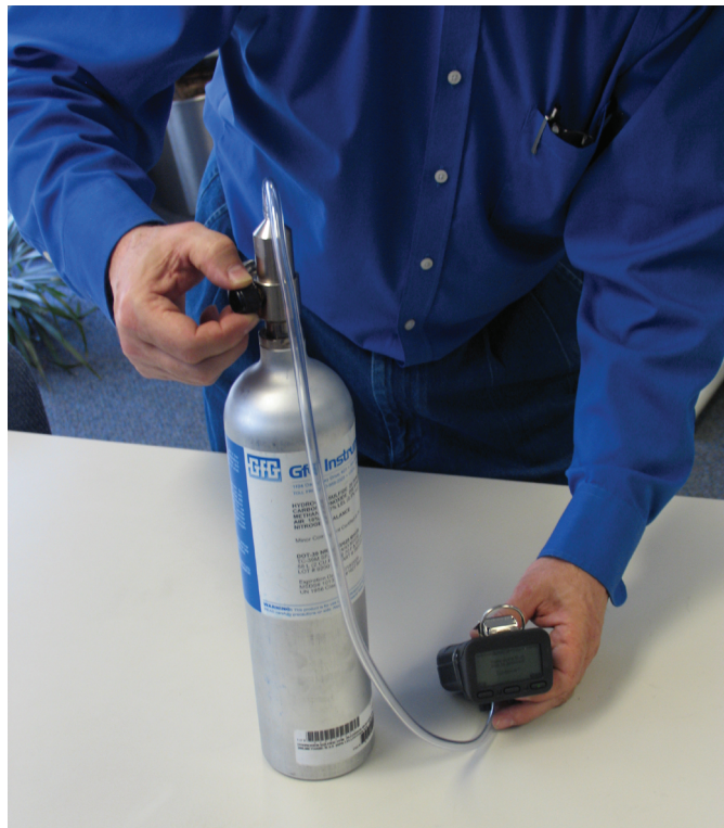
Figure 1: Performing a functional "bump test" by exposing the instrument to test gas takes only a few moments perform.
