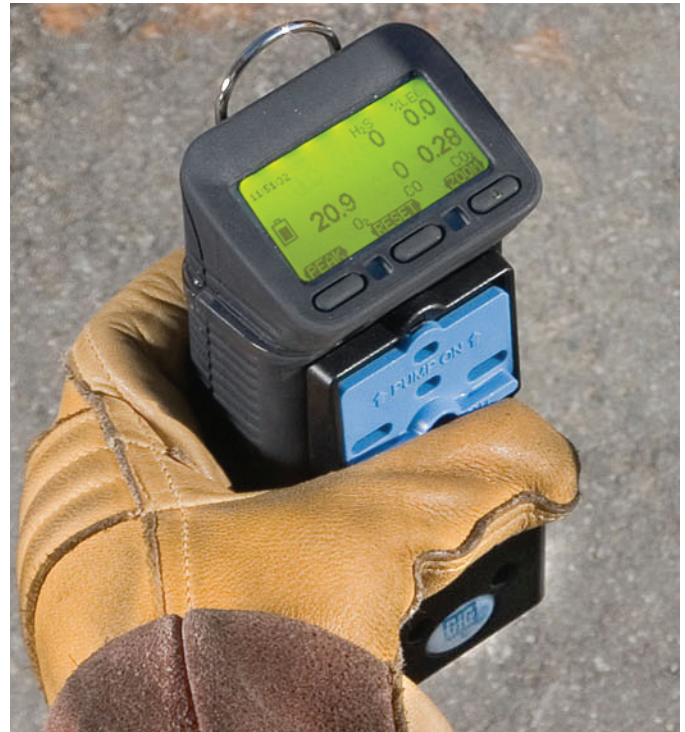
Figure 2: The only way to know whether an instrument is capable of proper performance is to expose it to test gas.
