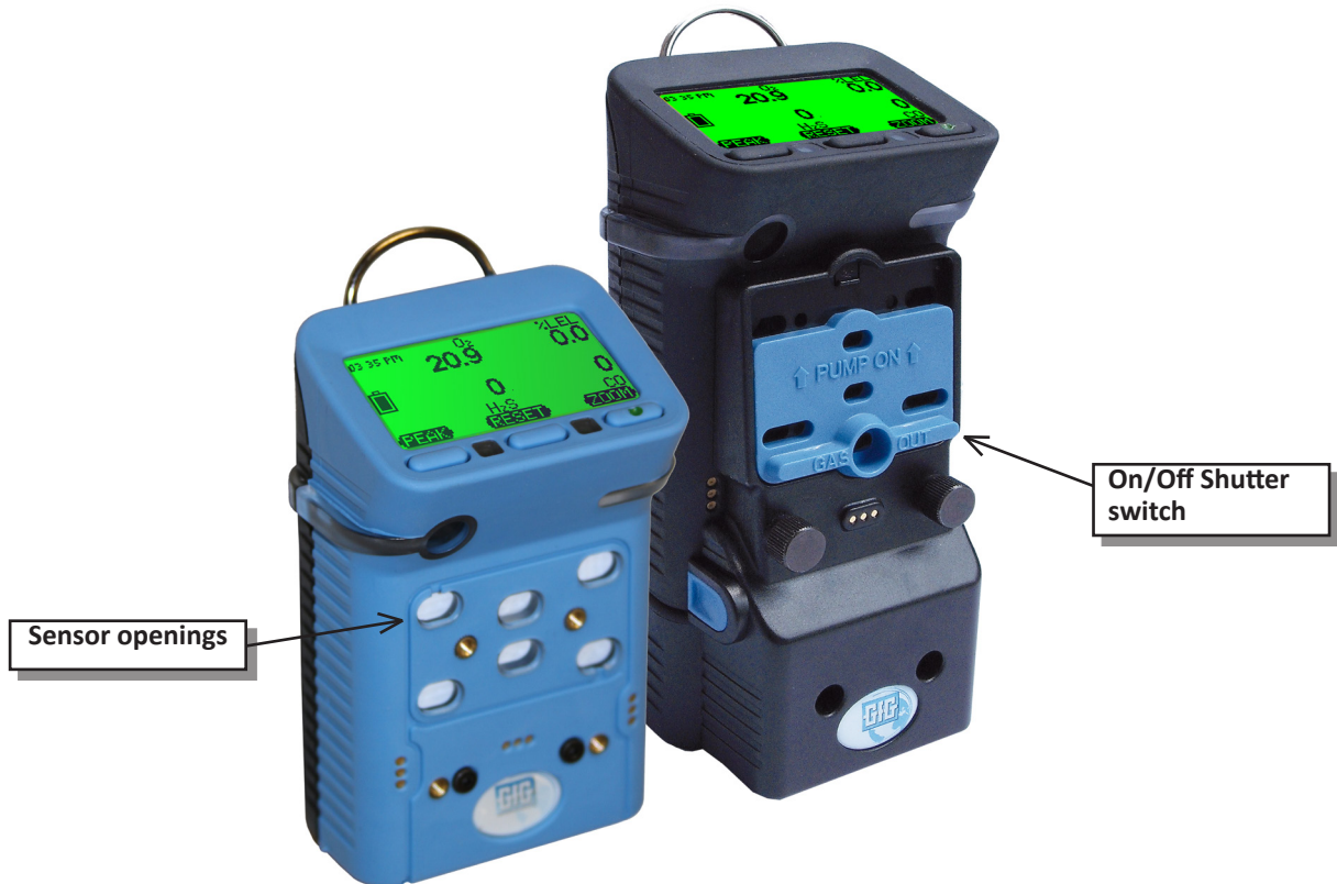
Figure 3: In diffusion operation the atmosphere reaches the sensors by diffusing through openings in the instrument housing. The openings are protected by moisture barrier filters. “Attachable” motorized pumps are physically secured to the instrument. A shutter switch permits operation of the in either “diffusion” or “sample-draw” mode.
