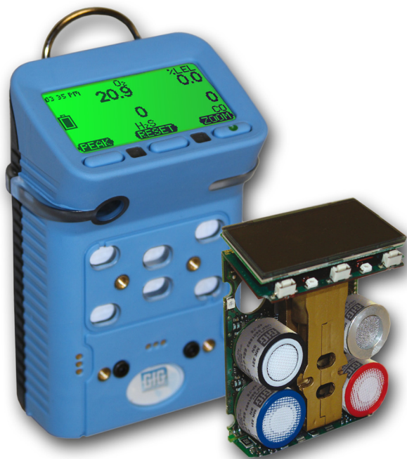
Figure 2: Portable confined space instruments can measure up to seven atmospheric hazards at the same time. Besides standard O 2 , LEL, CO and H 2 S sensors, the instrument can be equipped with IR combustible gas, PID, IR CO 2 , and a wide variety of substance-specific electrochemical toxic gas sensors.
